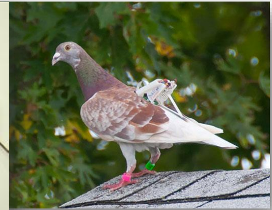
Piezoelectric material generates energy from the motion of a bird's wings in flight. (Michael Shafer, NAU)
