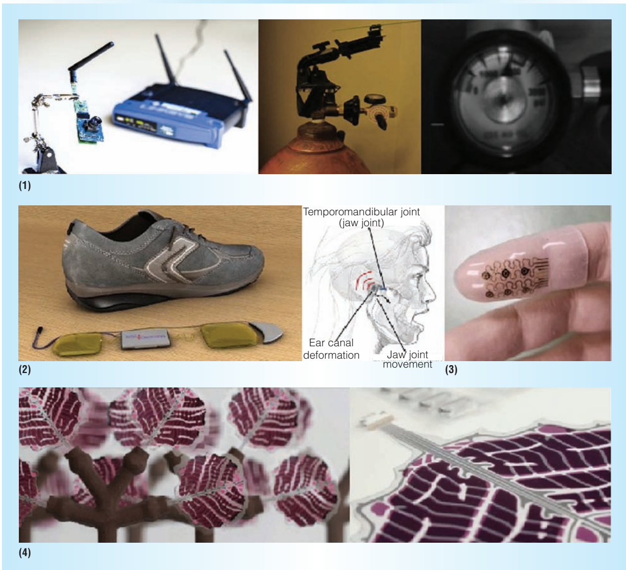
Figure A. A sampling of energy-harvesting Internet of Things devices. (1) A Wi-Fi-powered camera, with demonstration system mounted on an industrial gas cylinder, monitoring a pressure gauge. 7,8 (2) In-shoe piezoelectric devices 9 and a piezoelectric ear canal motion energy harvester. 10 (3) Thermoelectric generator. 11 (4) Solar leaves. 12
