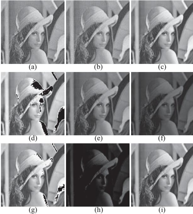
Figure 8. Gaussian filter results comparison. (a), Lenna grey scale 128\*128, as inputs to NEMSIP. (b), Matlab results. (c), NEMSIP result. (d), Larger input scale. (e), Smaller input scale affects darkness. (f), Larger scale of gate voltage affects output to be darker. (g), Smaller scale of gate voltage affects output quality. (h), high-speed results, with other setups same as (c). (i), high-speed mode with adjusted voltage scales.
