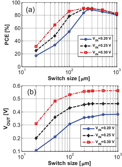
Fig. 9. Switch width optimization for the proposed HTFET charge pump with 300 pF  $C_p$ : (a) PCE; (b)  $V_{OUT}$ .
