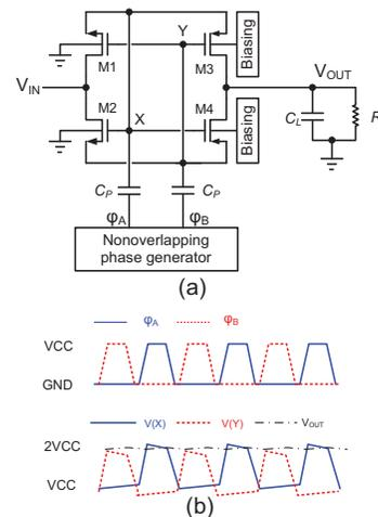
Fig. 1. A conventional cross-coupled charge pump.
