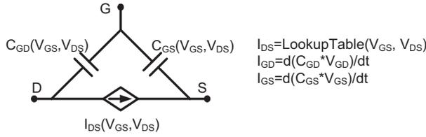
Fig. 4. HTFET circuit-level Verilog-A model [19][21].
