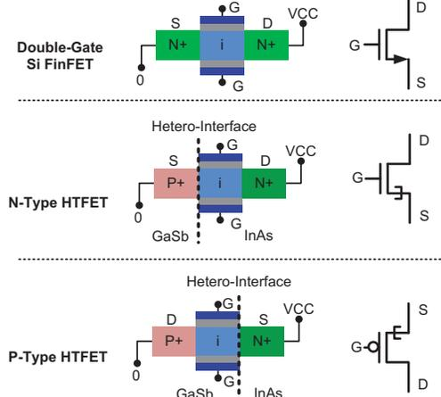
Fig. 2. Device structure and circuit symbol of N-type Si FinFET, N-type HTFET, and P-type HTFETs [18].
