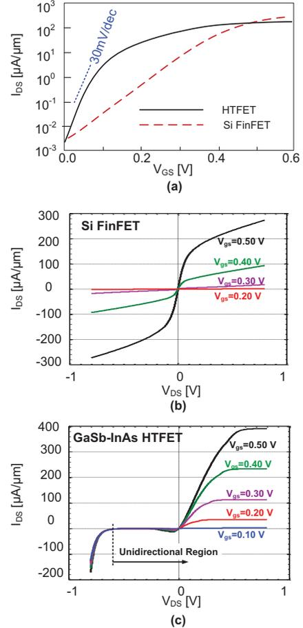
Fig. 3. Comparisons between Si FinFET and HTFET [18][20][23]. (a) Subthreshold slop comparison; (b) Si FinFET  $I_{DS}$ - $V_{DS}$  curves; (c) HTFET  $I_{DS}$ - $V_{DS}$  curves showing unidirectional tunneling current conduction.
