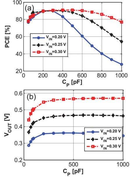
Fig. 8.  $C_p$  optimization of the proposed HTFET charge pump with 250  $\mu\text{m}$  switch width: (a) PCE; (b)  $V_{OUT}$ .
