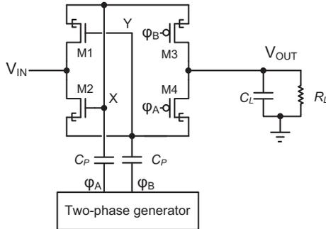
Fig. 5. Proposed cross-coupled HTFET charge pump.
