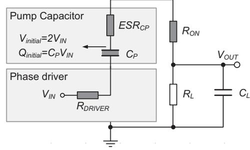
Fig. 6. Equivalent simplified circuit of the charge pumps in Fig. 1 and Fig. 4.
