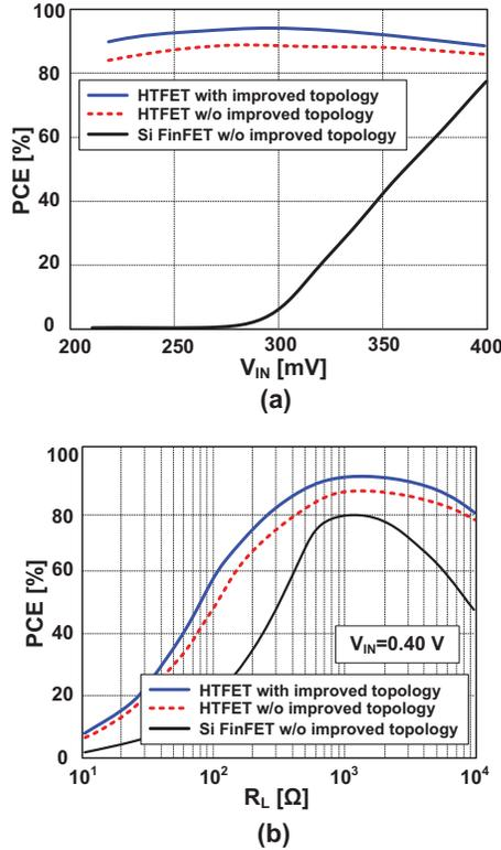
Fig. 10. Performance comparisons: (a) PCE versus  $V_{IN}$  with  $R_L=1.0$  k $\Omega$ ; (b) PCE versus  $R_L$  with  $V_{IN}=0.40$  V.
